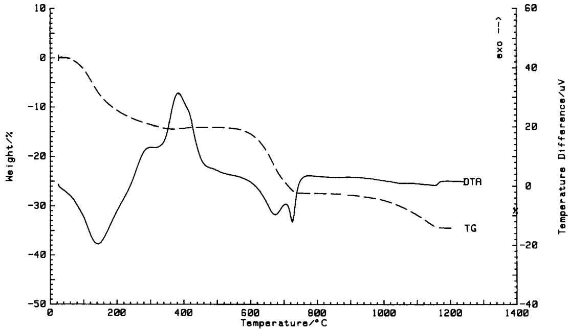
Fig. 2. Differential thermal analysis and thermogravimetry of lithium metazirconate powder produced from alkoxide precursors: route (a).
